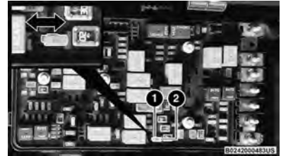
Power Outlets Fuse Locations
