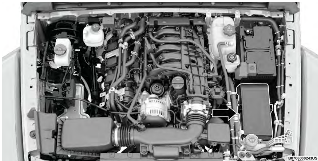
Power Distribution Center Location
