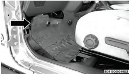
Front Carpet Pulled Away
