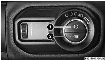
Fog Light Switch Location
