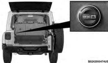
Rear Cargo Power Outlet
