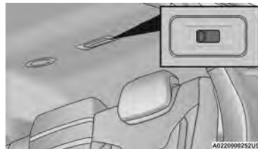
Rear Air Conditioning Control Switch
