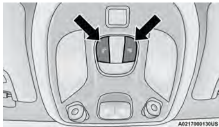
Overhead Light Switches
