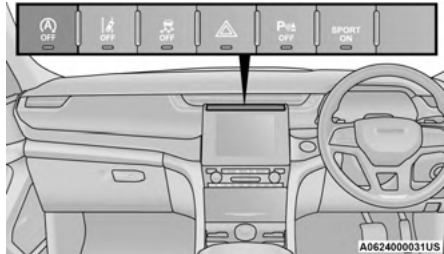
Stop/Start OFF Switch
