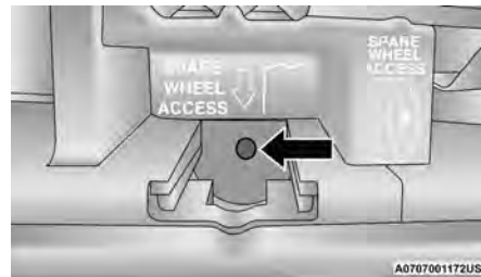
Winch Drive Nut Location
